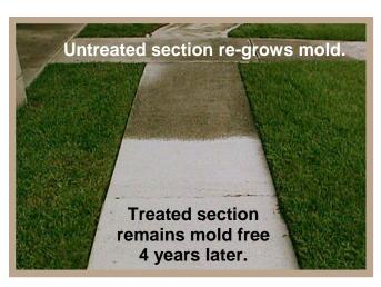
**TEST** – First Coast MicroGuard, Inc., long-time customer of Adsil, wanted to test the veracity of the third-party testing laboratory results of ASTM G-21, as posted on Adsil's web site. So the sidewalks leading into their offices were pressure washed to clean away the existing black mold growth, then, sections of the sidewalk were treated with MicroGuard Concrete Sealer and sections were left untreated.
